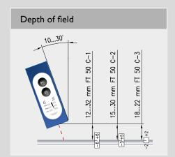
The depth of field of the FT 50 C also varies depending on the light spot geometry:
