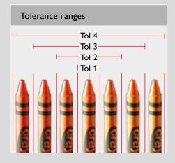
The detection window can be adapted by adjusting colour selectivity.
