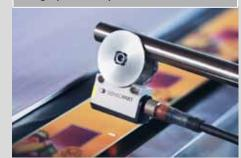
The FT 25-C miniature colour sensor reliably switches with 10 kHz with the taught-in colour (including black and white) and is particularly suitable for use in rapid processes, e.g. in labeling machines.
